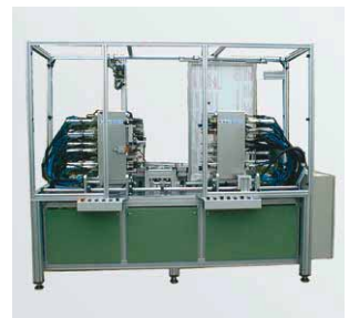
23 placing heads to assemble a computer chassis
