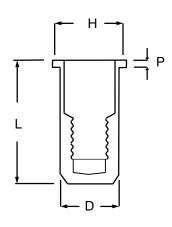
Steel inserts are supplied zinc plated and CR3 passivated. All plating materials are RoHS/WEEE compliant.
