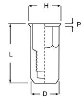
Steel inserts are supplied zinc plated and CR3 passivated. All plating materials are RoHS/WEEE compliant.
