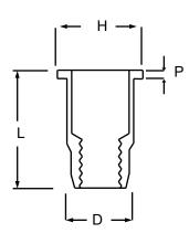
Steel inserts are supplied zinc plated and passivated. All plating materials are RoHS/WEEE compliant.
